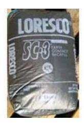
Loresco SC-3 has a bulk density of 1185 Kg per cubic meter. The fixed carbon content is greater than 99.35% by weight. The bulk density and high fixed carbon content coupled with the assured low resistivity medium allows for longer groundbed life at a lower operating cost.
